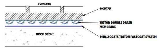
IF ROOF DECK IS CONCTETE AND RUNS TO A FALL - DIRECT APPLICATION ADVISED IF ROOF DECK IS BLOCK AND BEAM - A SCREED TO FALLS SHOULD BE LAID FIRST.
