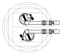
Single or dual outlets/discharge can be specified
