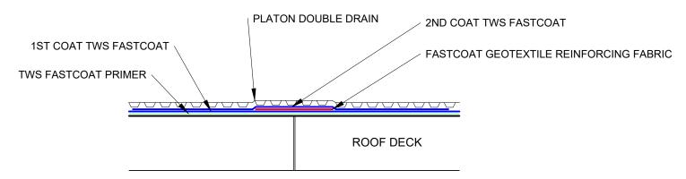
\* SUBSTRATE COULD BE SCREED, CONCRETE, OLD STABLE ASPHALT OR EXTERIOR GRADE PLYWOOD LAID OR FORMED TO A FALL AWAY FROM THE BUILDING
