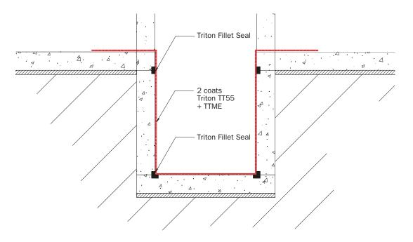
TRITON TT55 TO MASONRY WALLS + WALL/FLOOR DETAIL
