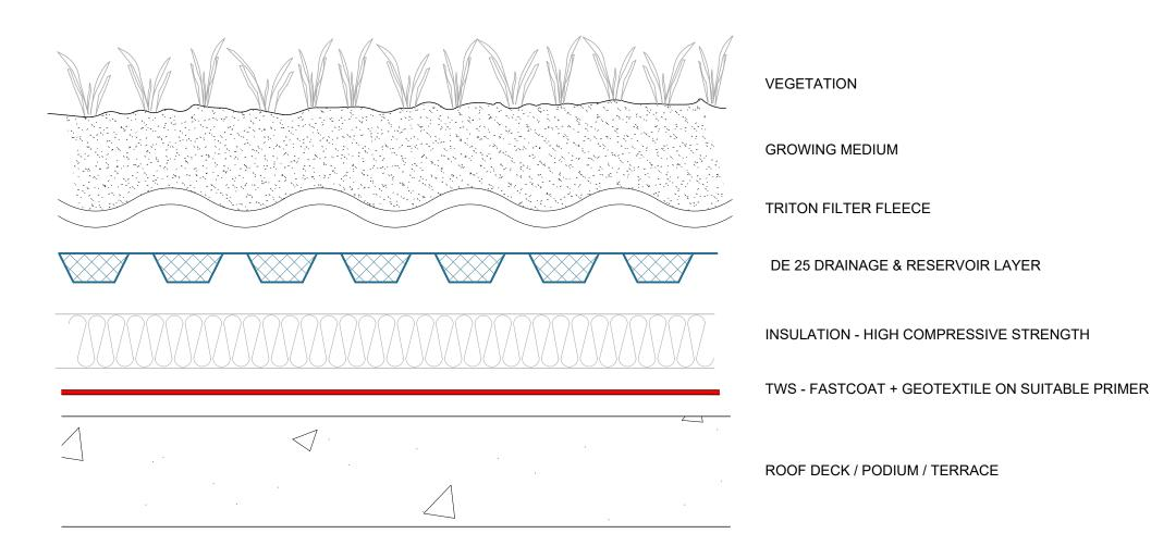
\* SUBSTRATE COULD BE SCREED, CONCRETE, OLD STABLE ASHPHALT OR EXTERIOR GRADE PLYWOOD
