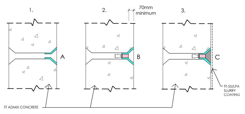
TIE BOLT CONES TO BE REMOVED
