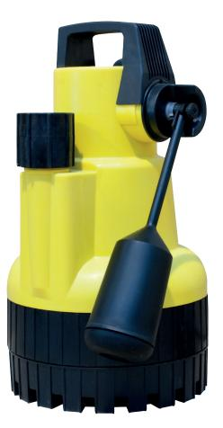
The state of the art Triton 303 is designed to give top performance and achieve high levels of efficiency thanks to optimised hydraulic systems and motors. The pump is fitted with a magnetic float switch with variable level control and maximum travel stop. A locking disk enables straightforward adaption of the pump to external control systems. Supplied free standing for quick installation.
