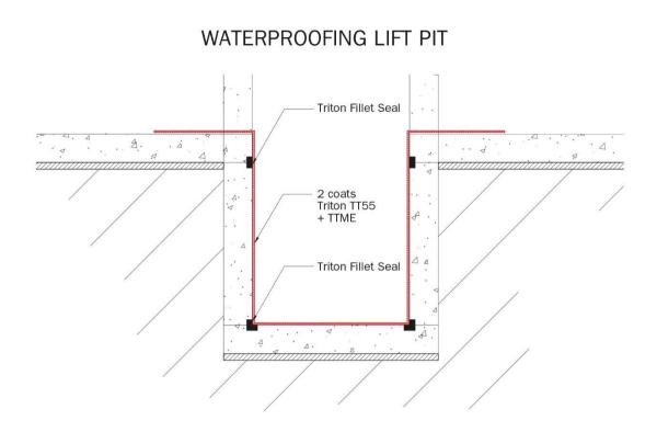
TRITON TT55 TO MASONRY WALLS + WALL/FLOOR DETAIL
