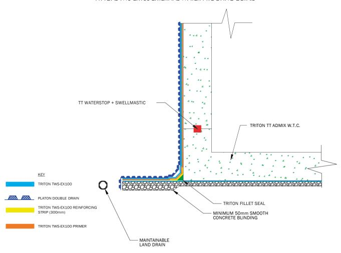
For installation advice please refer to separate application guidelines available from Triton Systems. Overlaps are 50mm edge over edge and 100mm end over end. End laps should be staggered to avoid an excessive build up of layers in one area. TWS EX Primer LT would normally be used before EX100 is applied.
