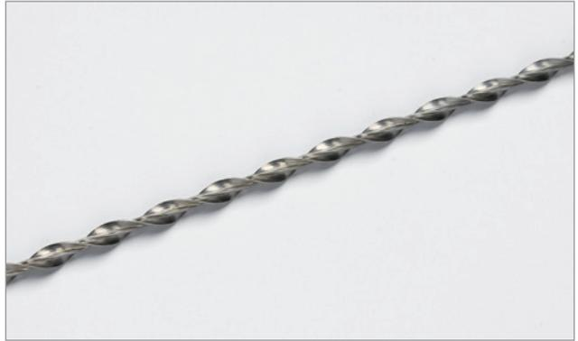
Stainless steel Tribar Rods are designed to stabilise existing masonry and are used in general crack stitching repairs, to reinforce masonry above failed lintels, as a method of overpinning to reduce the underpinning load and to re-tie solid or cavity masonry panels. Typical applications will be in buildings with shallow foundations or which are subject to movement, masonry arches and bridge repairs.
