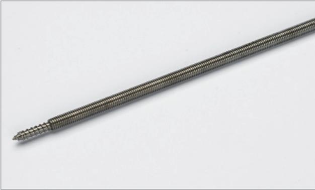
Typically used to stabilise old or bowed walls, Triton's Lateral Restraints are manufactured from 8mm diameter 304 austenitic Stainless Steel rods. They are available in a standard 1m length but can be supplied in other lengths on request. The restraints are designed to restrain the whole of the brick outer structure to the floor joists and offer important benefits:
