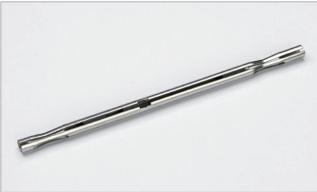
A high quality 10mm stainless steel tie for use in situations that require both the inner and outer wall to be anchored with resin. The 'waisted' ends give the tie a mechanical and an adhesive fixing once the resin is applied. Suitable for use in brick, lightweight block, timber and mortar. The AA10 tie is available in lengths to suit varying cavity widths and construction types. An inbuilt feature enables load tests to be carried out on site on the inner leaf if necessary.
