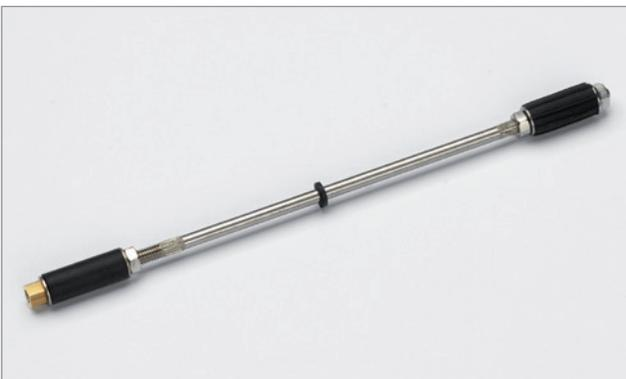
Manufactured from stainless steel and Neoprene, the 11mm EE10 tie features a torque nut which sets both the inner and outer expanders independently. The EE10 tie is particularly suitable for brick or stone structures where there is a sound inner leaf and in constructions of four stories or less. Can be pull tested.
