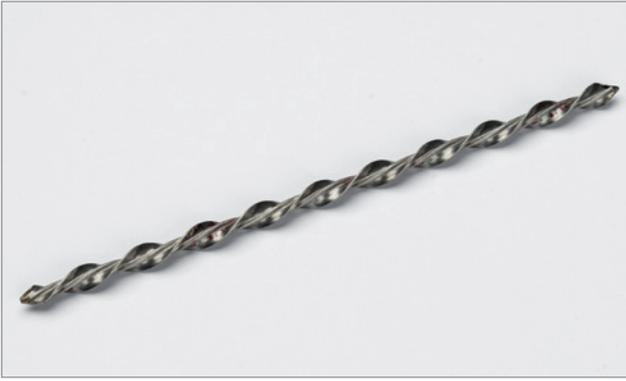
A helical dry fix replacement wall tie for use where both outer and inner leaf is of good sound quality. Quick and easy to install, the one-piece Dryfix tie requires no resin, grout or mechanical expansion. Suitable for pinning masonry features, it can be used in bricks, blocks, concrete, hard mortar and timber. The Dryfix tie can be installed through insulation without affecting thermal performance. Manufactured from stainless steel.
