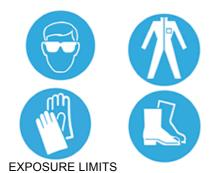
Wear goggles or face shield, PVC or synthetic rubber gloves, protective footwear, and overalls.
