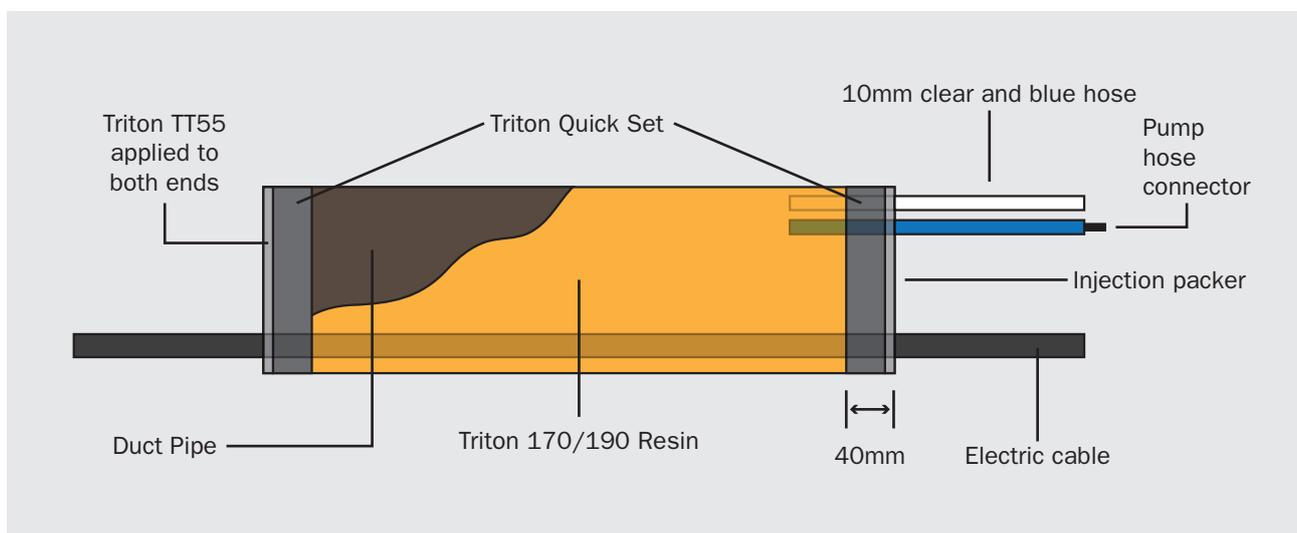
4. Once the Triton Quick Set has set, inject Triton 190 through the blue inlet hose until resin flows freely through the clear plastic tube.
